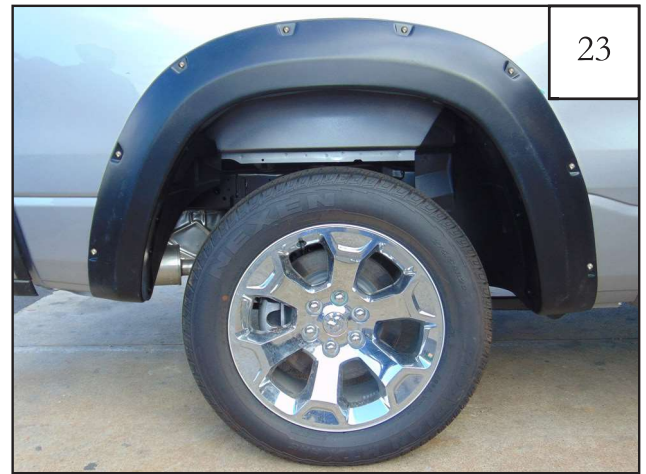
Completed rear flare installation.
