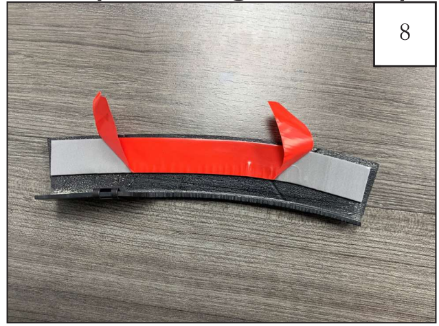
For model years 2022+ vehicles, peel back 2 inches of tape on supplied inner bracket - If older than 2022 – proceed to Step 12
