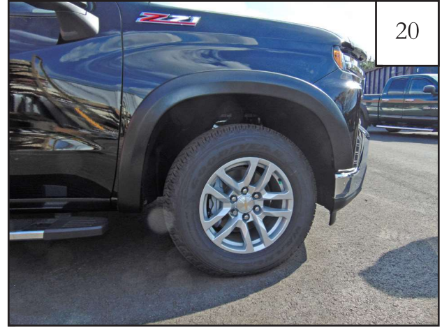
Completed front flare installation.
