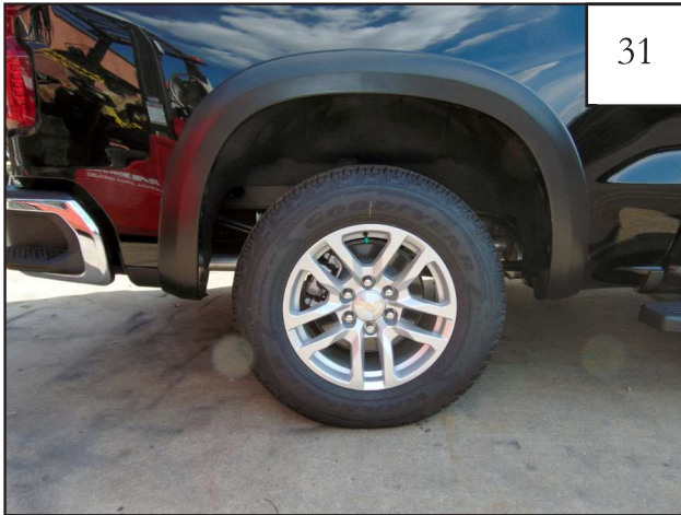
Completed rear flare installation.
