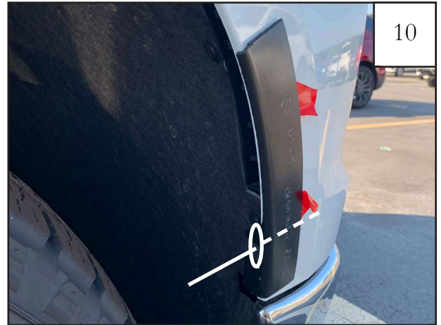
Line up the U-clip hole on the inner bracket to the mark made in Step 5 and install the inner bracket.
