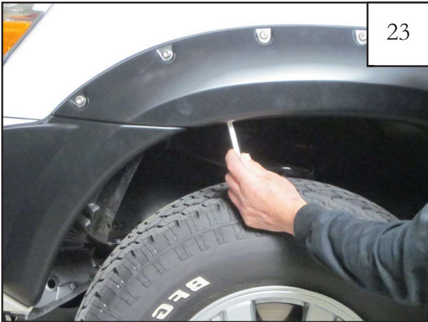
Install a supplied Phillips Truss Screw (SW1-0050) through holes in flare and into Clips installed in Step 21
