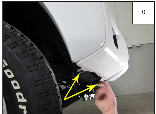
Remove two factory screws underneath the the front bumper cover.
