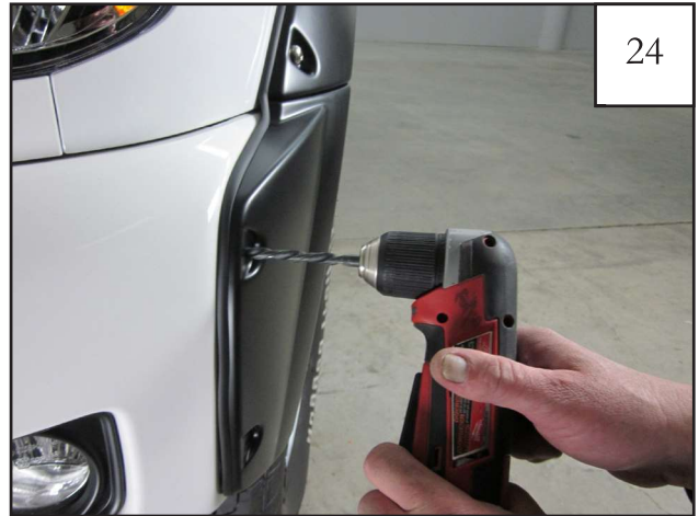
Drill through holes in bumper piece and into sheet metal with a 5/16" drill bit
