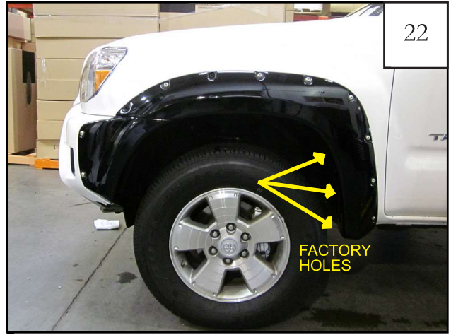
Reposition flare on fender and install three 20mm hex screws (SW1-0036) through holes in flare and into factory holes
